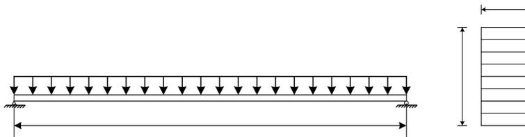
Fig. 5 Glulam Girder Subjected to Distributed Load
