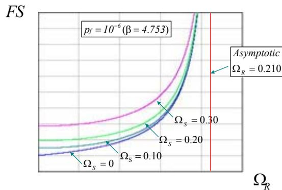
Fig. 2 Relationship between  $\Omega_R$ ,  $\Omega_S$  and  $FS$  for  $p_f = 10^{-6}$
