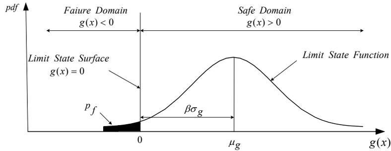
Fig. 1 Relationship between Safety Index and Failure Probability
