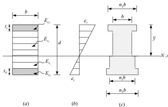
Fig. 4 Sandwiched Girder: (a) Typical Cross-Section; (b) Transformed Section.
