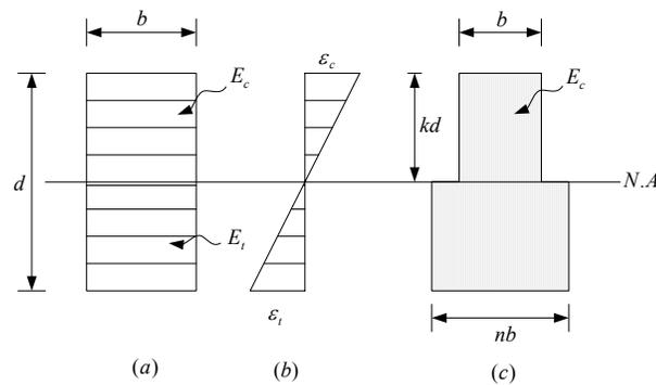
Fig. 3 Glulam Girder: (a) Cross-Section; (b) Transformed Section.
